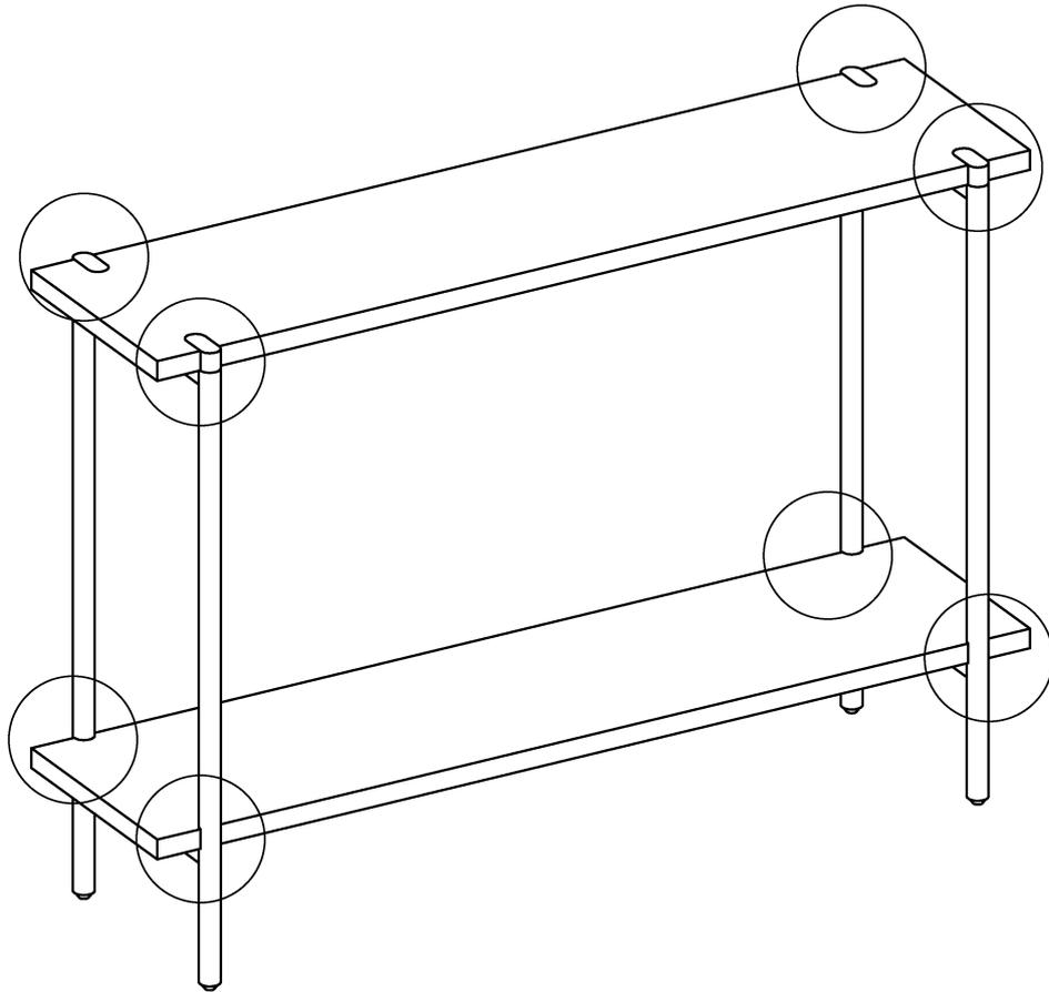
After checking all gaps and ensuring they are even, please tighten bolts fully.
