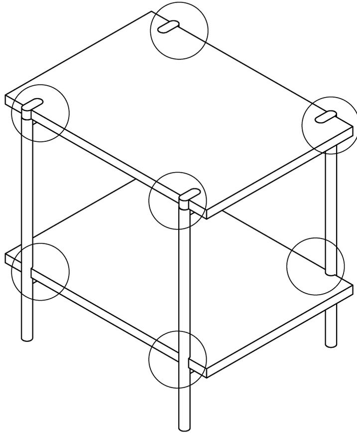
After checking all gaps and ensuring they are even, please tighten bolts fully.
